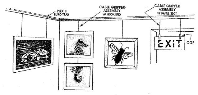
Architecturally compatible, satin finished, anodized aluminum **EURO-TRAK** mounts securely to wall, accommodating any wall width. Ball-end cables glide smoothly along TRAK for exact wall-towall positioning.
